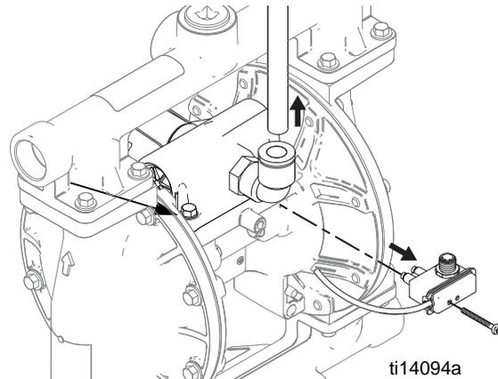
**FIG. 1. Reed switch assembly and air line removal**
