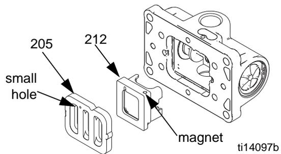
**FIG. 6. Air valve cup and plate installation**
