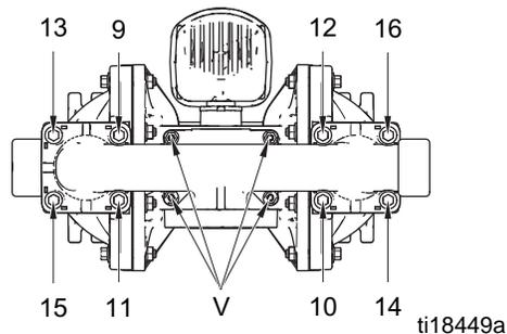
**FIG. 10. Torque sequence**
