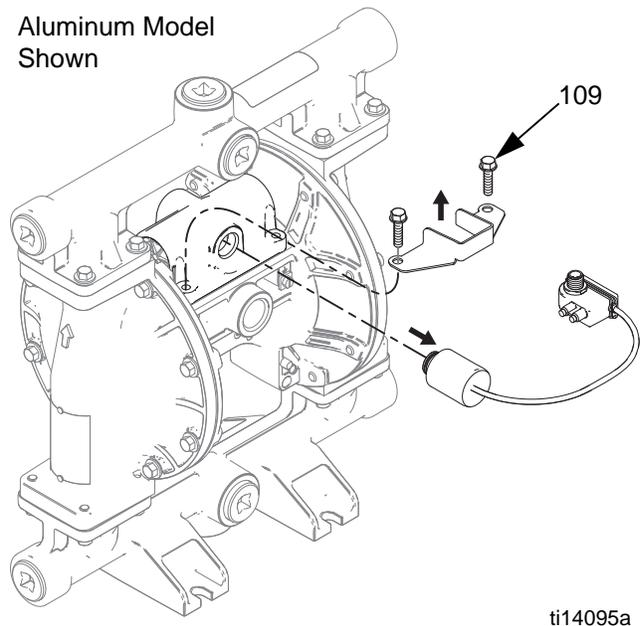
**FIG. 2. Solenoid removal**
