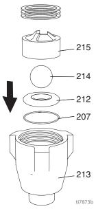
11. Place intake valve (213) assembly in vice. Install cylinder (205) assembly to intake valve. Torque to 350 ft-lb (475 N•m).
