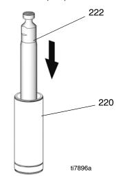
5. Grease top inch or two of piston rod (222) that will go through the cylinder throat packings.
