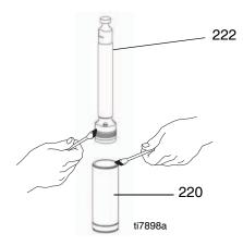
4. Carefully slide piston rod assembly (222) into top edge of sleeve (220).
