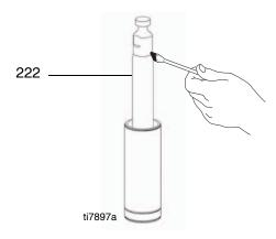
6. Grease o-ring (207) and place on sleeve. Slide one o-ring (207) inside cylinder (205). Slide sleeve/piston rod assembly (222) into bottom of cylinder.
