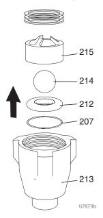
3. Select proper ball travel for material sprayed. Reassemble as shown.
