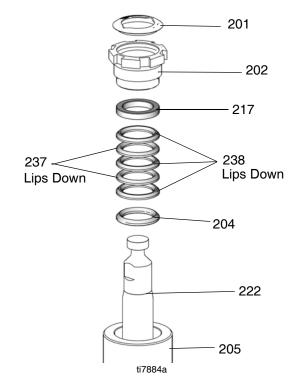
10. Reassemble intake valve (213) as shown.
