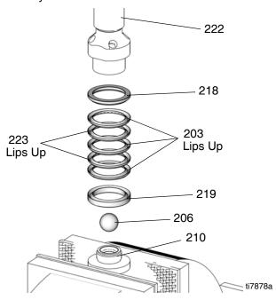
Clean all parts with a compatible solvent and inspect them for wear or damage. Replace any worn parts.
