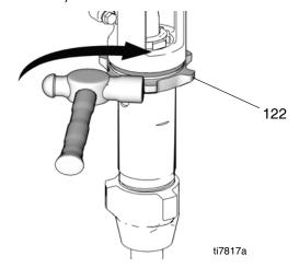
15. Install coupling (125) around pump rod.
