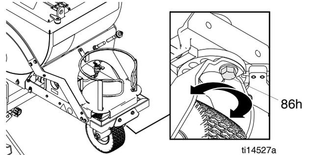
2. Rotate front wheel fork left or right, as necessary, to straighten alignment.
