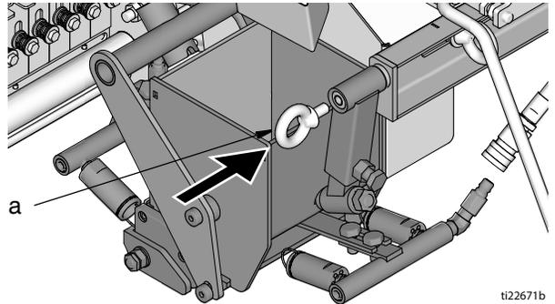
4. Attach spring loaded handle (Z) to the yoke (31) and turn 90 degrees to lock into place.
