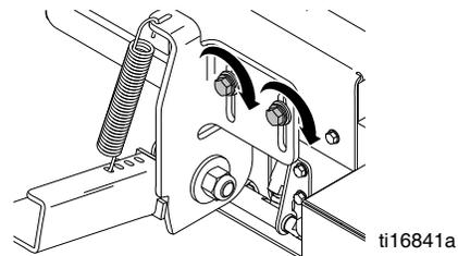
4. Spring position may be moved to a different hole. The farthest holes provide greatest force to close the gate.
