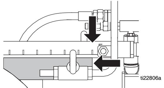
3. Tighten bolts (c) on screed box mounting bracket.
