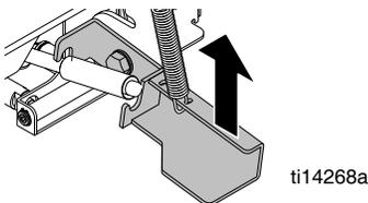
4. Align hole of rod clevis with connecting hole in screed box yoke and install hairpin cotter pin.
