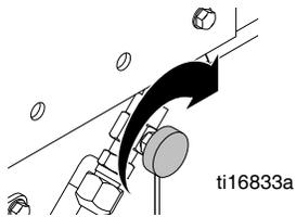
2. Slide screed box under screed shroud and press down on screed box lever.
