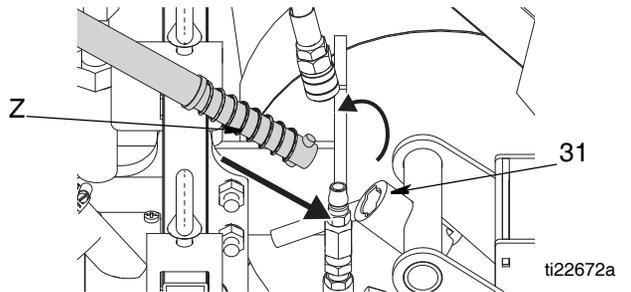
5. Attach both gas hoses to quick release couplings (10).
