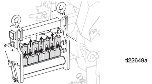
Bead flow rate can be adjusted using the Bead Flow Rate Lever on the outside of the Bead Dispenser Box.
