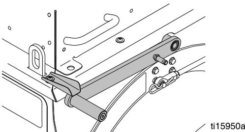
6. Load bag of thermoplastic directly on kettle heat exchanger. Close cover with cover latches.
