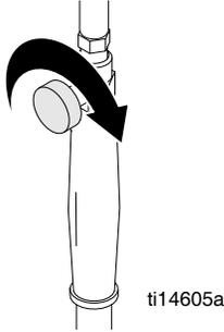
2. Close manual shut-off valve on propane tank when finished melting and heating thermoplastic material.
