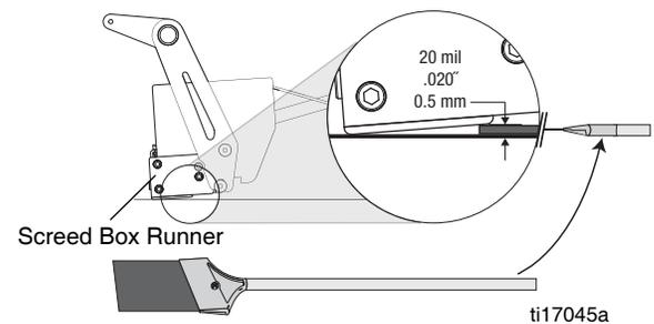
3. Tighten bolts on screed box mounting bracket.
