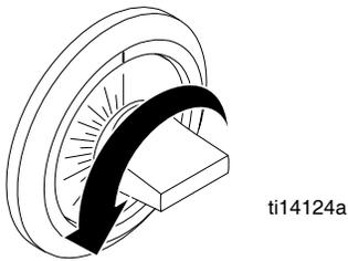
3. Fully close front and rear screed burner flow flame adjusting valve OFF.
