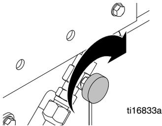
4. Close kettle manual shut-off valve.
