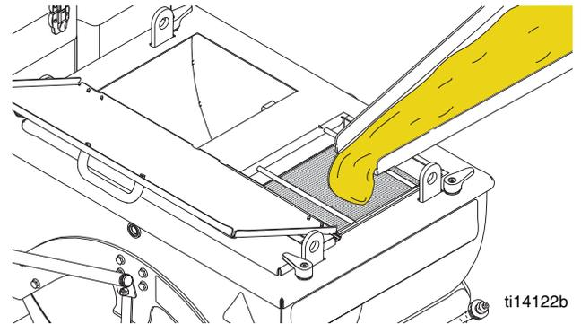
6. Move Gate Valve Actuator (S) to raised position and fill screed box with melted thermoplastic material.
