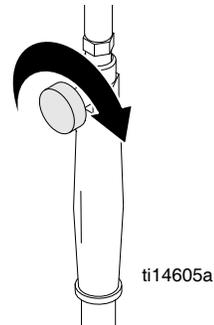
6. Turn main gas valve on propane tank OFF.
