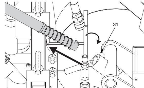
4. Remove bolt and slide FlexDie box off.
