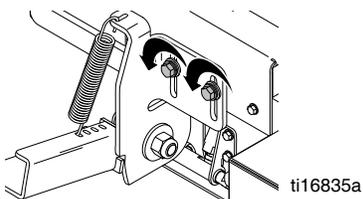
2. Slide mount down until leading box edge of screed box runner is just off of the ground surface. For best performance, raise leading edge .020 in. (0.5 mm) off ground surface. Scraper blade may be used to set this depth.
