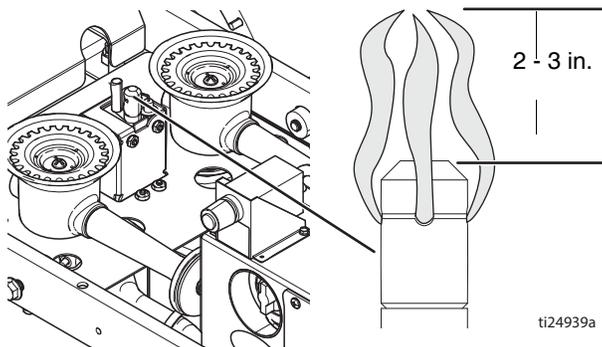
**DAILY:** Make sure LP-gas only flows to burner when safety shut-off valve knob is pressed in.
