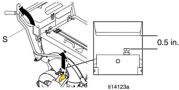
**NOTE:** The material gate is adjustable. The gate is factory set at a 0.5 in. (1.3 cm) gap. You can increase this gap for more material flow or decrease the gap for less material flow.
