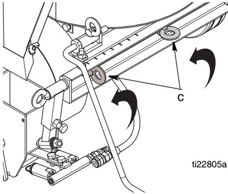
2. Slide mount left or right until edge of the frame is aligned with desired markings on bracket.
