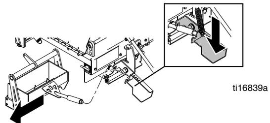
4. Disengage screed box rod from screed box lever and carefully remove screed box.
