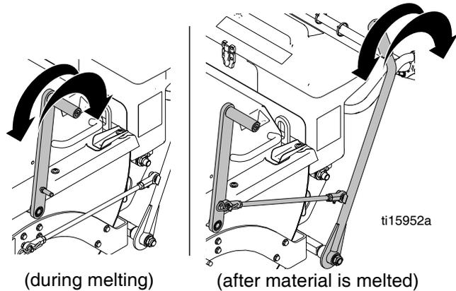
8. Repeat steps 5 - 7 until kettle is filled with melted thermoplastic.
