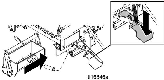
3. Engage screed box rod into screed box lever.
