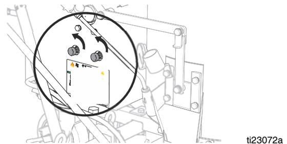
6. Place torch at end of screed box burners to ignite and use screed box burners flame adjusting valve to adjust to desired flame.
