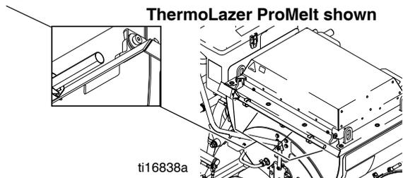
Check to make sure combustion air supply openings on kettle are not obstructed.
