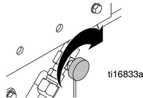
2. Remove hairpin cotter pin connecting screed box to rod clevis.
