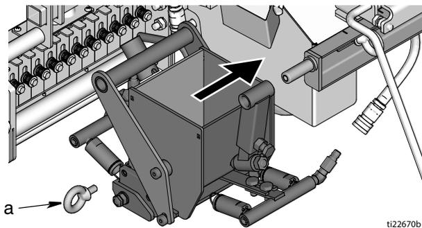
3. Replace and tighten bolt (a).
