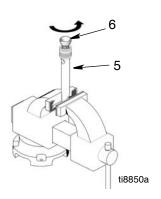
Remove packing and glands from piston rod. Note orientation for installation.
