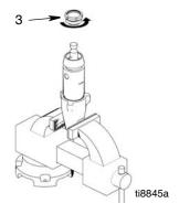
2. Unscrew intake valve from cylinder.
