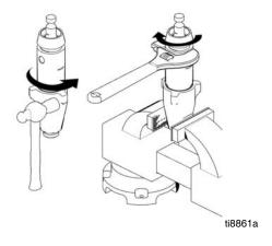
16. Torque packing nut to: 140 +/- 10 in-lb (15 +/- 1 N•m) 288467, 288468, 288819, 24M629.
