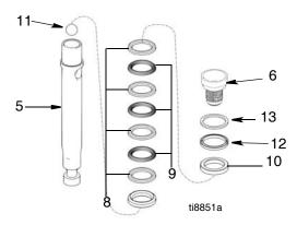
8. Remove throat packings and glands from cylinder. Discard throat packings and glands.
