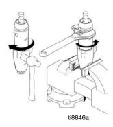
Disassemble intake valve. Clean and inspect o-ring (17). You may need to use a pick to remove o-ring.
