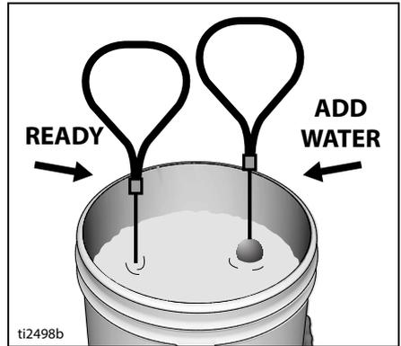
6. If the ball does not sink completely into the mixture within 10 seconds, add more water, agitate and try test again.
