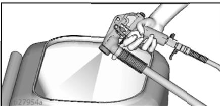
4. Trigger gun into waste pail until hopper no longer contains water and all water is removed from hose and pump system.
