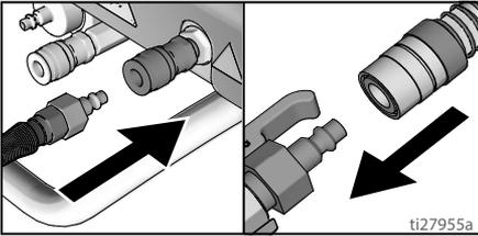
2. Connect one end of material hose to material outlet and the other end to gun material inlet. Firmly tighten connections.
