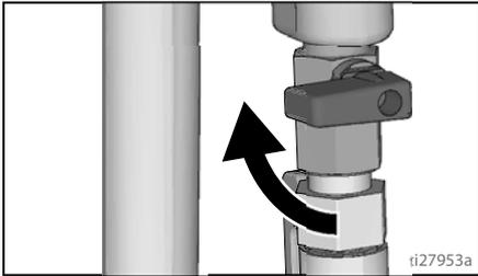
4. Open Prime Valve to start flow. Aim gun into hopper and trigger the gun.
