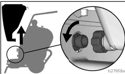
2. Lift material hopper straight up, off the unit.
