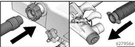
3. Install spray nozzle. See **Recommended Nozzle & Disc Selection Charts**, page 15. Pulling trigger when installing nozzle makes assembly easier.
