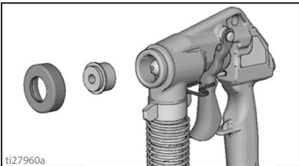
4. Open gun air control valve, forcing air through nozzle to clear out any remaining material.
