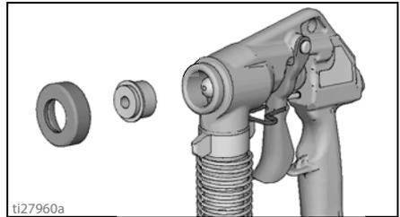
3. Open gun air control valve. Make certain prime valve is closed.
