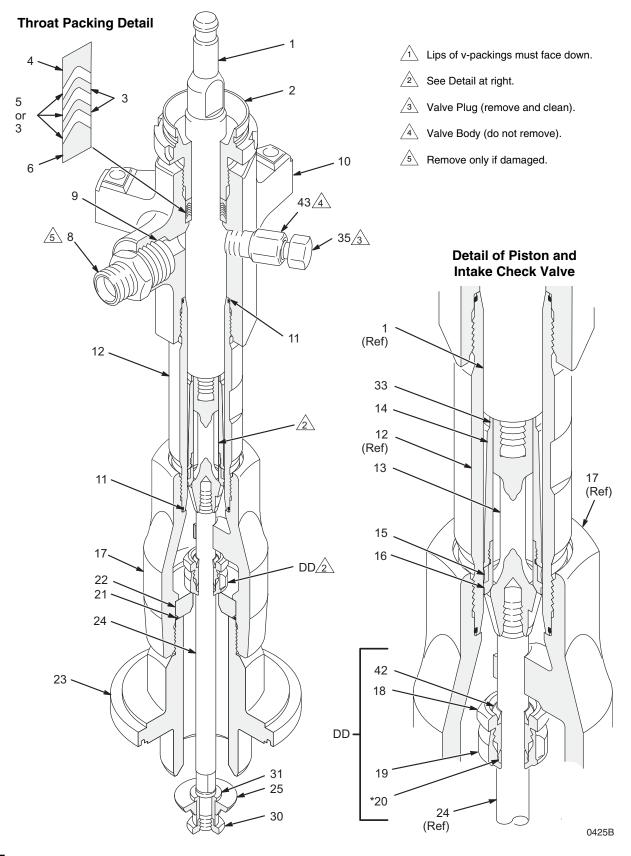
Place the flats of the piston seat (16) in a vise. Using a 13 mm (1/2 in.) dia. brass rod (EE), unscrew the piston guide (14) from the piston seat (16). See FIG. 6. Remove the piston seal (15); always replace with a new one. Inspect the mating surfaces of the piston (13) and piston seat (16) for nicks, scoring or wear.
