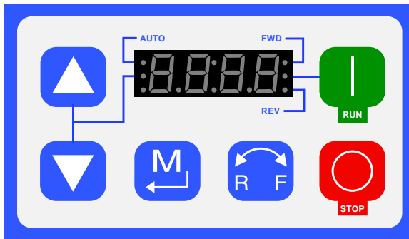
Figure 15 VFD Control Panel
